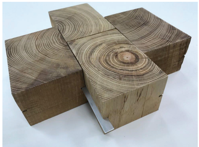
2 1/2" depth x 4" x 6" rectangular Black Locust pavers with aluminum spline for tongue and groove installation.
