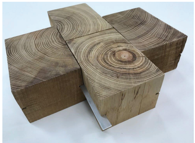
2 ½ depth x 4" x 6" rectangular Black Locust pavers with aluminum spline for tongue and groove installation.
