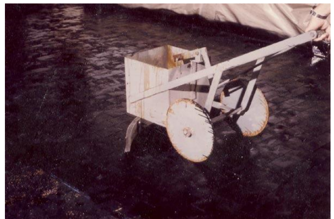
Squeegee Machine for coating application
