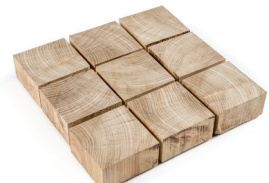
2" depth x 4" x 4" Black Locust pavers on mesh, in tile pattern, with 3/8" spaces.
